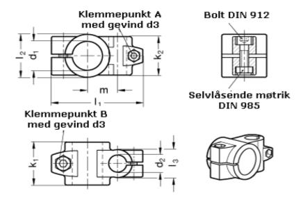
Adjustable clamp lever for d3 = GN 911-M10-55 have to be ordred separately Adjustable clamp lever for d4 = GN 911-M 8-32 have to be ordred separately d1 = 48= 30d2 = M10d3 = M 8d4 = 65
